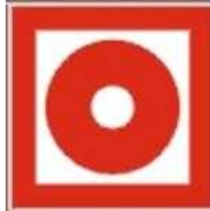
Fire alarm button
