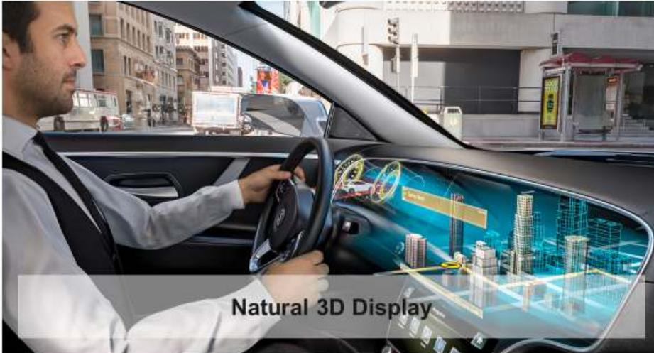
And that is not all. And then we are also profiting from our **technologies for the human-machine interface**. Example: animated displays. These are new systems that graphically show information in the driver's field of vision. In the picture you can see a large-area display. It is three dimensional. And it can be operated intuitively.
