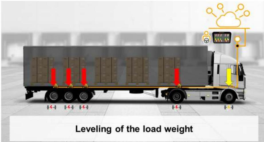
Our **electronic air-spring system is also intelligent**. We have expanded it with a kind of built-in scale, which constantly shows the load weight. It indicates if there is an overload. That helps the drivers. That helps the owners. Because the transport then complies with legal regulations. This makes traffic safer. And without overloads, trucks subject roads to less wear and tear.
